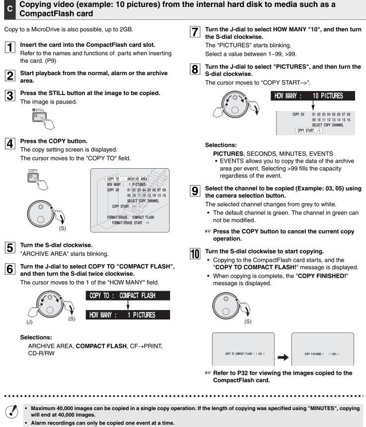
· Format the CompactFlash card (FAT16) using this equipment. Formats done using FAT 32 will not be recognized.
